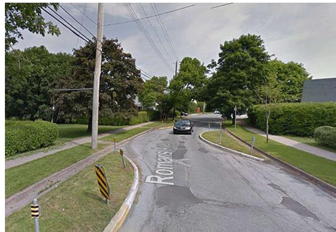
A chicane creates a horizontal deflection in the roadway. (Source: Google Street View)
