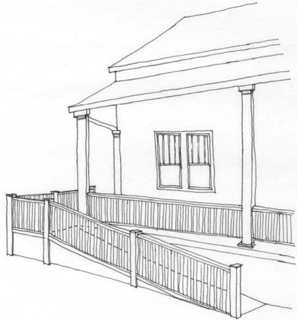
The design of this ramp is simple and rectangular, similar to the historic detailing on the house.
