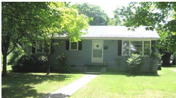
The house at 1323 Adams Street displays a window arrangement typical of the Ranch style: a wide inner window flanked by narrower operable windows.
