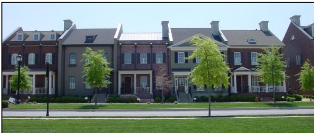
Figure 5-29: These attached residential structures demonstrate how different materials, changes in wall planes, offsets, projections, recesses, and other architectural techniques can promote variety in building façades.
