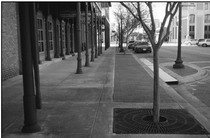
Figure 5-87: When planted within tree pits, street trees need sufficient room for water absorption and root growth.
