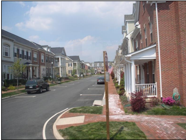
Figure 5-129: Narrow streets are more attractive to pedestrians, reduce stormwater runoff, and minimize maintenance costs.
