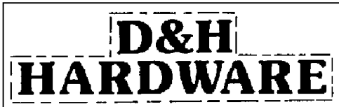
Figure 5-136: Sign area is determined by drawing a box (indicated by the dashed line) around all type and markings associated with the sign.
