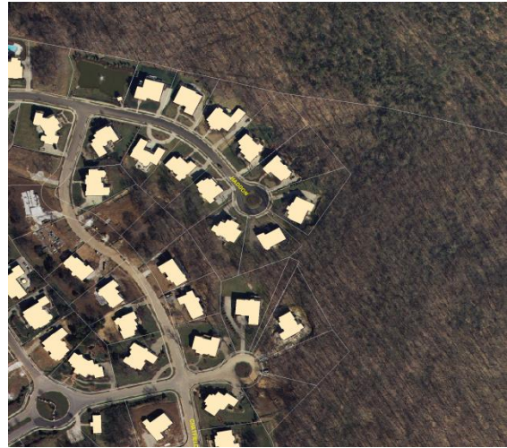
Figure 5-130: Cul-de-sacs are most appropriately used in areas of steep topography and where stream crossings are prohibited, as shown in this image.
