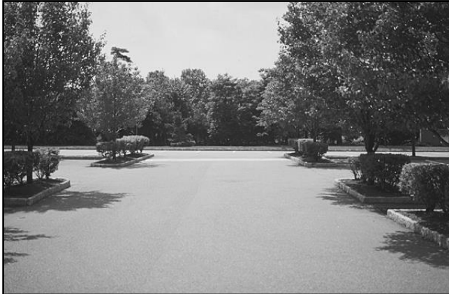
Figure 5-81: Larger surface parking lots can be visually divided up into a series of smaller parking areas through the use of lengthwise landscaped islands.
