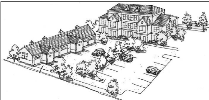
Figure 5-33: Garages serving attached residential structures must be oriented perpendicular to the primary streets serving the development to minimize their visual impact.
