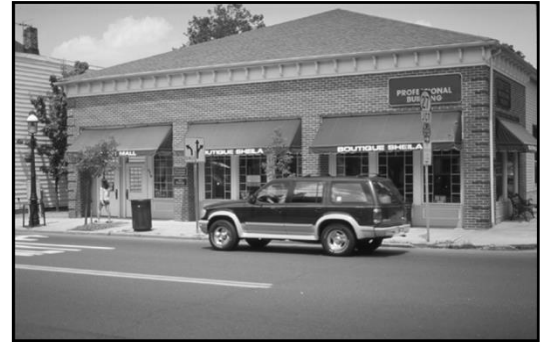
Figure 5-34: Buildings are more pedestrian-oriented when primary entrances are located adjacent to the sidewalk or street instead of to surface parking lots.
