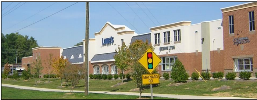
Figure 5-48: The mass of large-scale development can be made more human-scaled and pedestrian-friendly through the use of techniques like liner buildings or architecture replicating liner buildings as depicted here.
