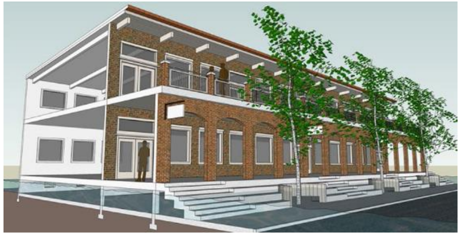
Figure 3-17. Conceptual model of low-rise nonresidential building above the Base Flood Elevation, along the southern half of the block.
