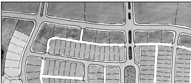
Figure 5-18: Rear alleys can be used as an alternative to reverse frontage lots.
