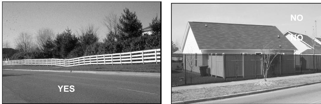
Figure 5-17: The image on the left demonstrates appropriate screening for reverse frontage lots. Fences or walls without landscape are inappropriate.
