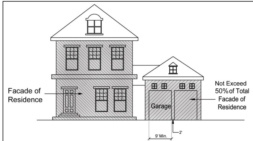
Figure 5-21: This diagram illustrates the size of a street-facing garage relative to the dwelling unit façade size.
