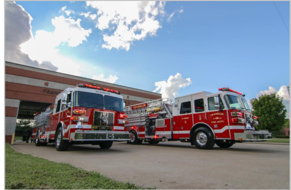
Ladder 8, the new apparatus for Station 8, arrived in 2015, along with Ladder 5. The two identical trucks are 2015 Sutphen SA75 Quint Aerial ladder trucks, which cost $790,576.55 per truck.
