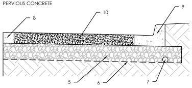
PERVIOUS CONCRETE INSTALLATION SHALL BE PERFORMED PER ACI 522.1-13: SPECIFICATION FOR PERVIOUS CONCRETE PAVEMENT.
