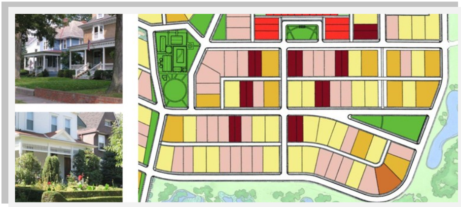
Figure 15. A plan of a typical lot distribution, where lot types repeat within a block and facades must be varied. (Different colors indicate different house models.)
