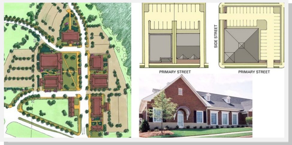
Figure 13. This illustration shows a sample master plan drawing, surface parking options, and a photographic example of a typical nonresidential lot.
