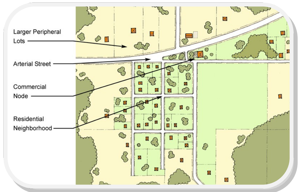
Figure 1. Hamlets are traditionally located at major intersections and include residential and limited commercial development organized within a grid-street pattern supplemented with generous amounts of open space.
