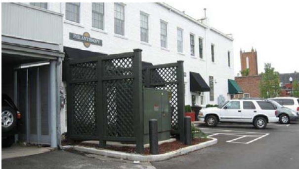
The occupants at 432 Main Street appropriately located electronic and waste-disposal equipment on the rear elevation and screened it with fencing.
